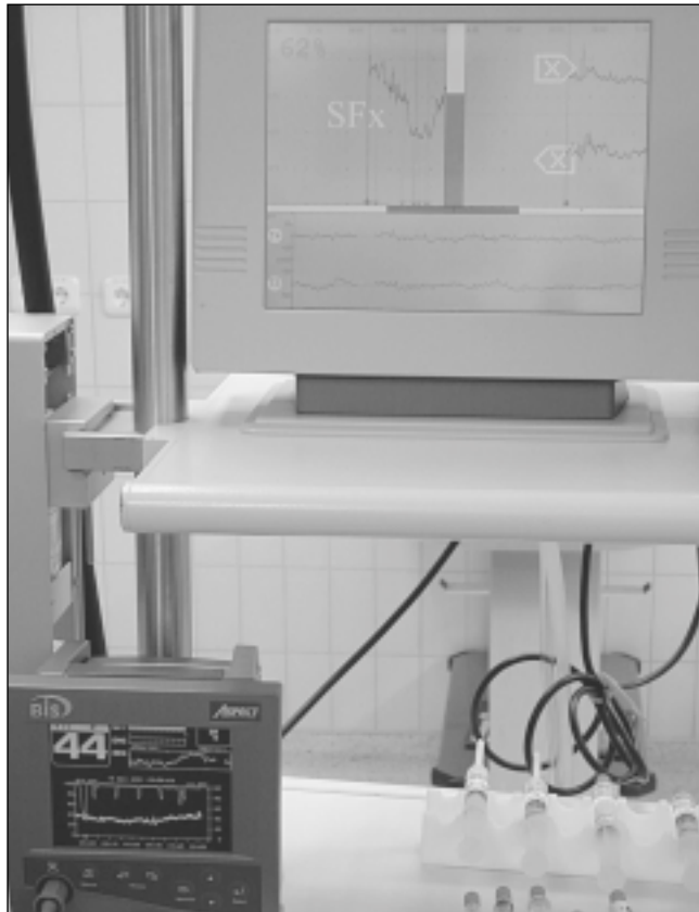
Fig 1. Picture comparing graph on PSM 2000 and BIS CABG surgery, intermittent cross clamping technique, balanced anaesthesia, note temperature drifts on PSM 2000 – no drift on BIS.
